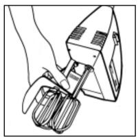
outward from the front of the Mixer. (Figure C) Snap the Attachment onto the Beater shafts.
